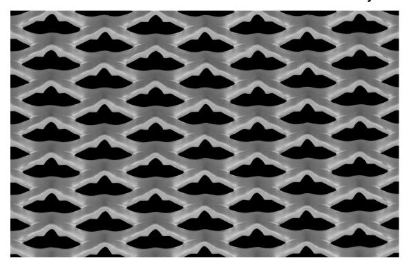
LW Pitch:38.10mmStrand Width:4.75mmSW Pitch:13.85mmThickness:2.50mmWeight:13.40 kg / m2Open Area:29%
